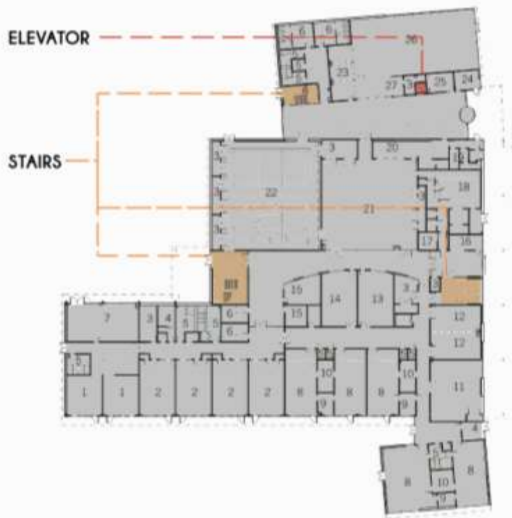
Fig. 5.1.1.5. Ground Floor Vertical Circulation
