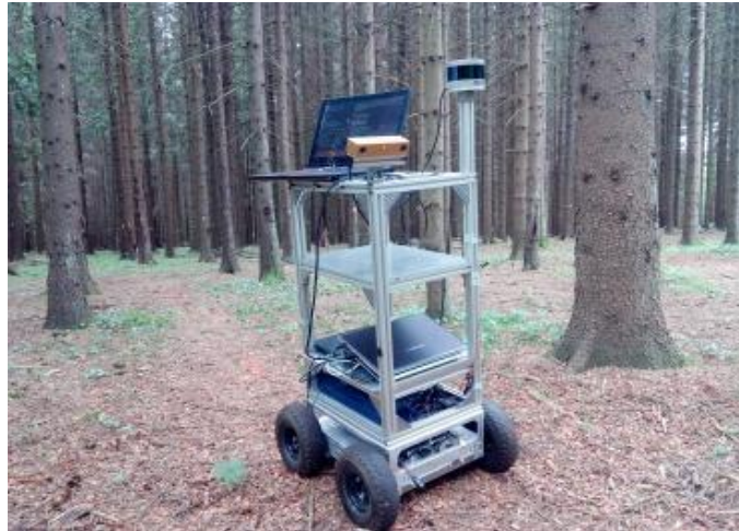
Figure 17: Four-wheeled rover Superdroid 4WD IG52 DB [27].
