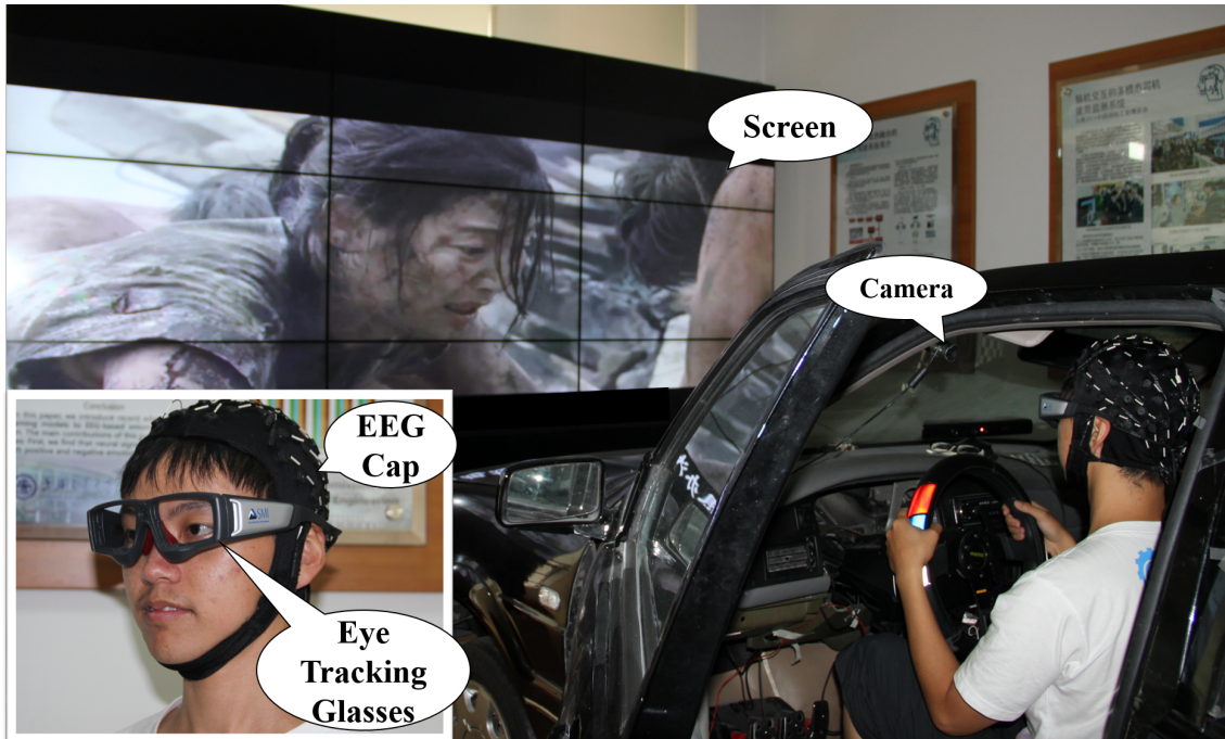
Figure 4.1: Arrangement for 62 Channel EEG Brain Wave Acquisition in Brain-like Computing and Machine Intelligence Laboratory, Shanghai Jiao Tong University. [Source: seed dataset description page ]
