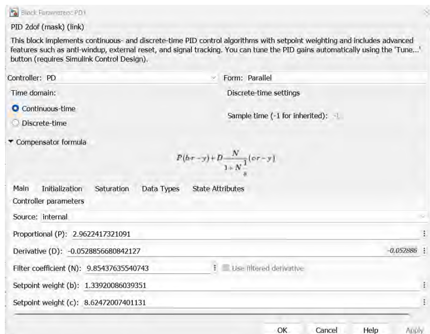
Fig.4.32. Parameter Block of Proportional-Derivative (PD) Controller
