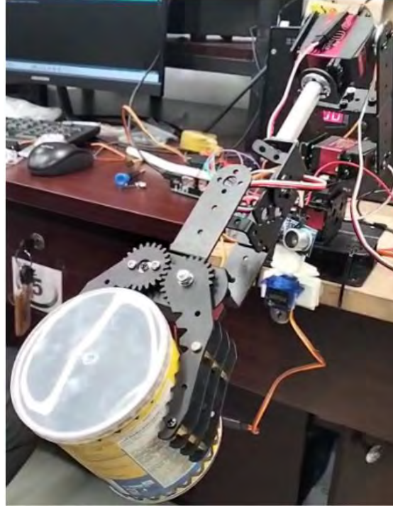
Fig.5.1 Completed Arm Structure
