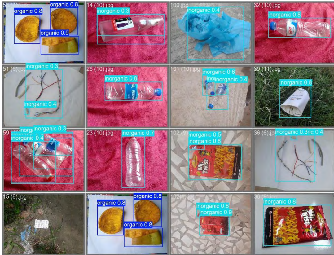
Fig.4.26. Recognized waste by YOLOv8n
