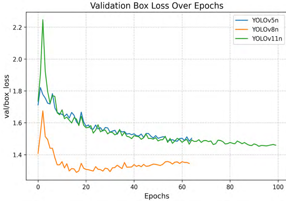
Fig.4.17. Validation Box Loss Over Epochs for YOLOv5n, YOLOv8n, YOLOv11n.
