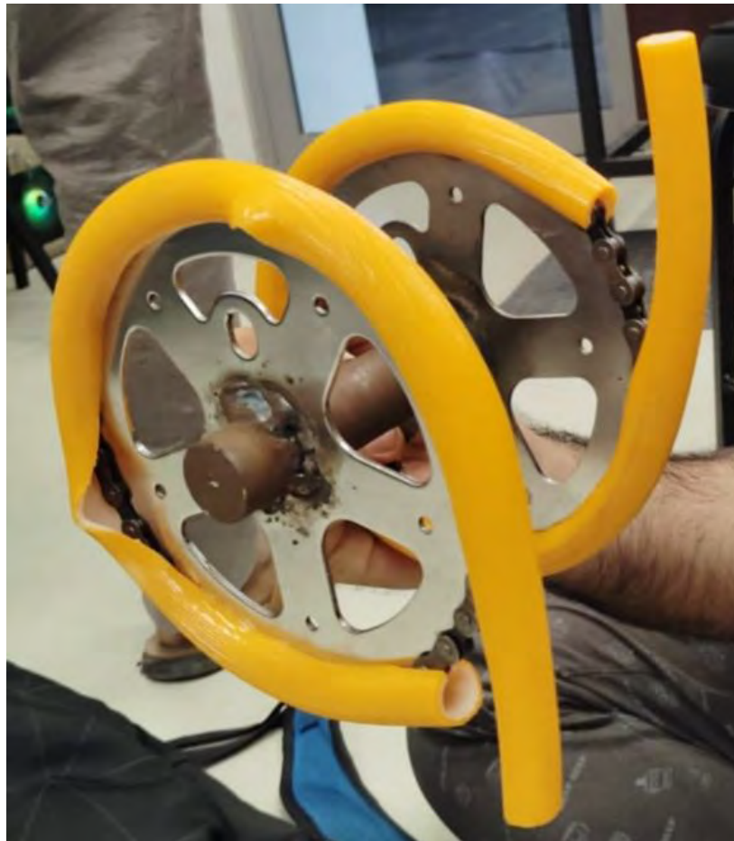
Fig.5.6 Gas cylinder pipe being wrapped around the wheel
