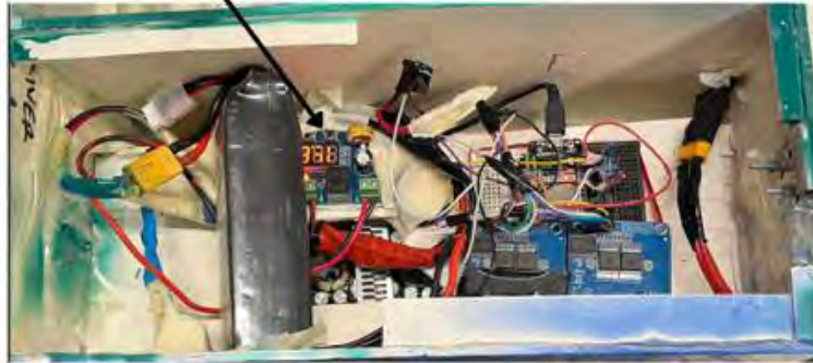
Fig.5.13 Over Discharge Protection Circuit
