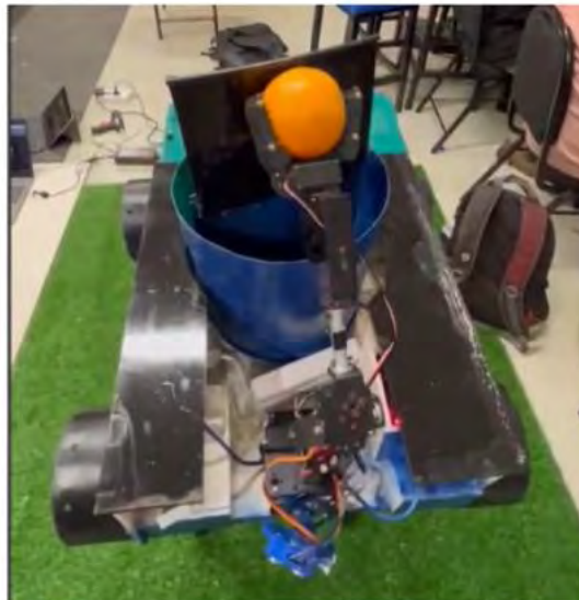
Fig.5.18 Picking of biodegradable waste and dumping it in the respective bin
