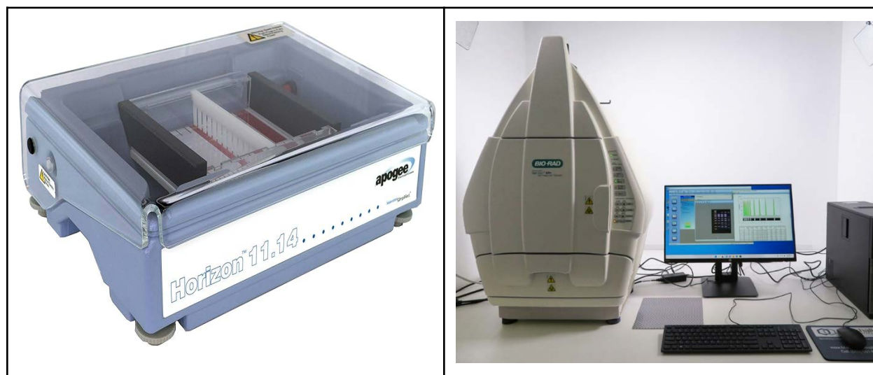
Fig. 3.6.2: Apogee Gel apparatus and Biorad Gel Doc for electrophoresis and visualization
