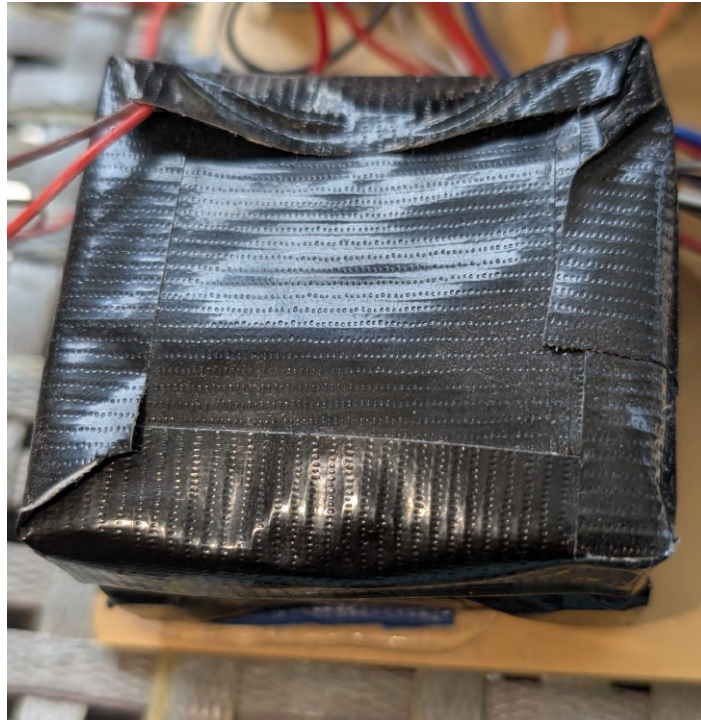
Figure 39: Car battery: 3.7V ( \approx 4V ), 1000mah - 3 batteries, total 11.6V ( \approx 12V )
