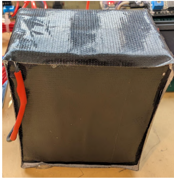
Figure 40: Station battery: 3.6V ( \approx 4V ) 2600 mah - 6 batteries, total 21.6V ( \approx 24V )
