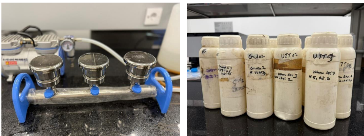
Figure 4: Sample processing of E. coli through membrane filtration
