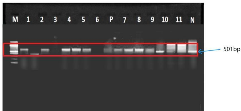
Figure 28: Agarose gel electrophoresis of PCR assay of blaVIM gene. Here M lane is 100 bp DNA marker, and lane (1-11) are some positive samples band at 501 bp.
