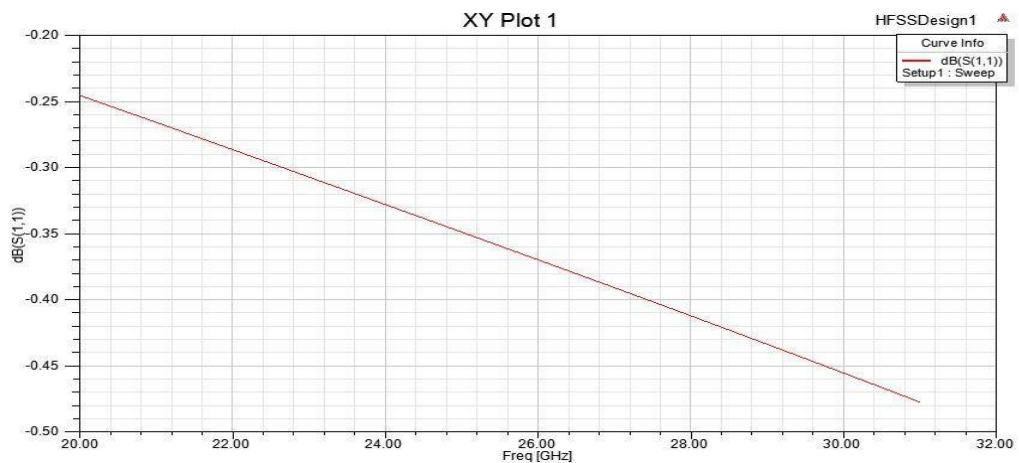
Fig 22a: S Parameter for 1x1 circular patch antenna
