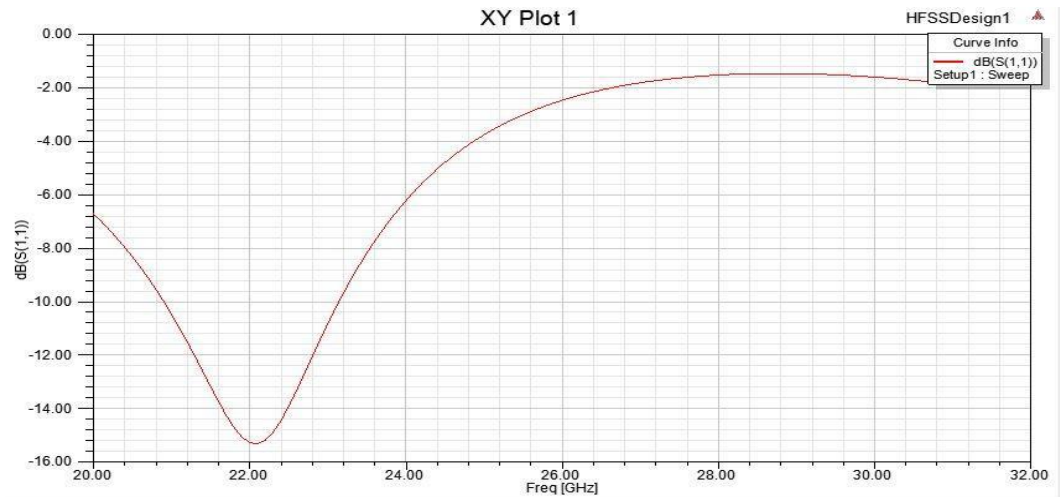
Fig 23a: S Parameter for 1x1 circular patch antenna
