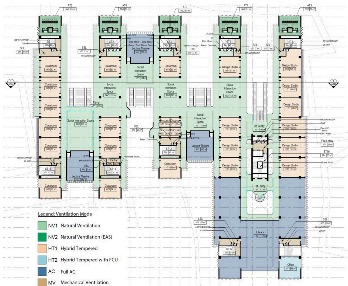
Figure 4.1.G: Ventilation of Brac University (Source: www.transsolar.com )
