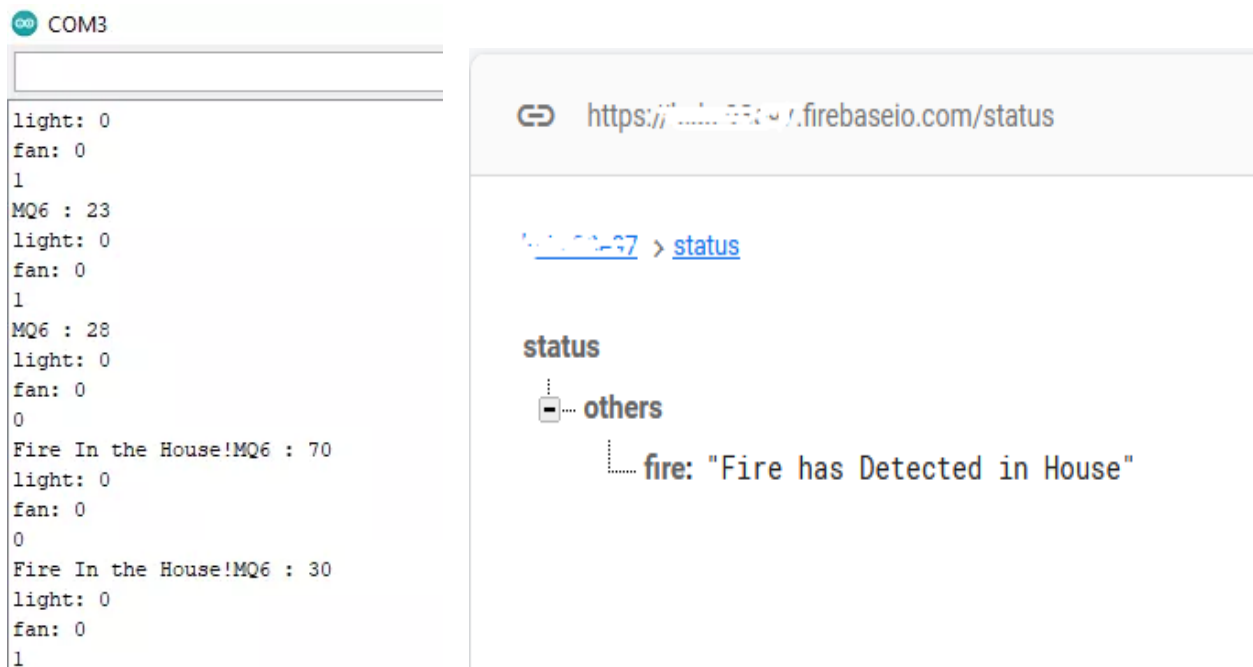
Figure 5. 8: Sensor testing of prototype design (Flame Sensor)
