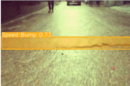
Figure 6.37: Speed bump segmentation
