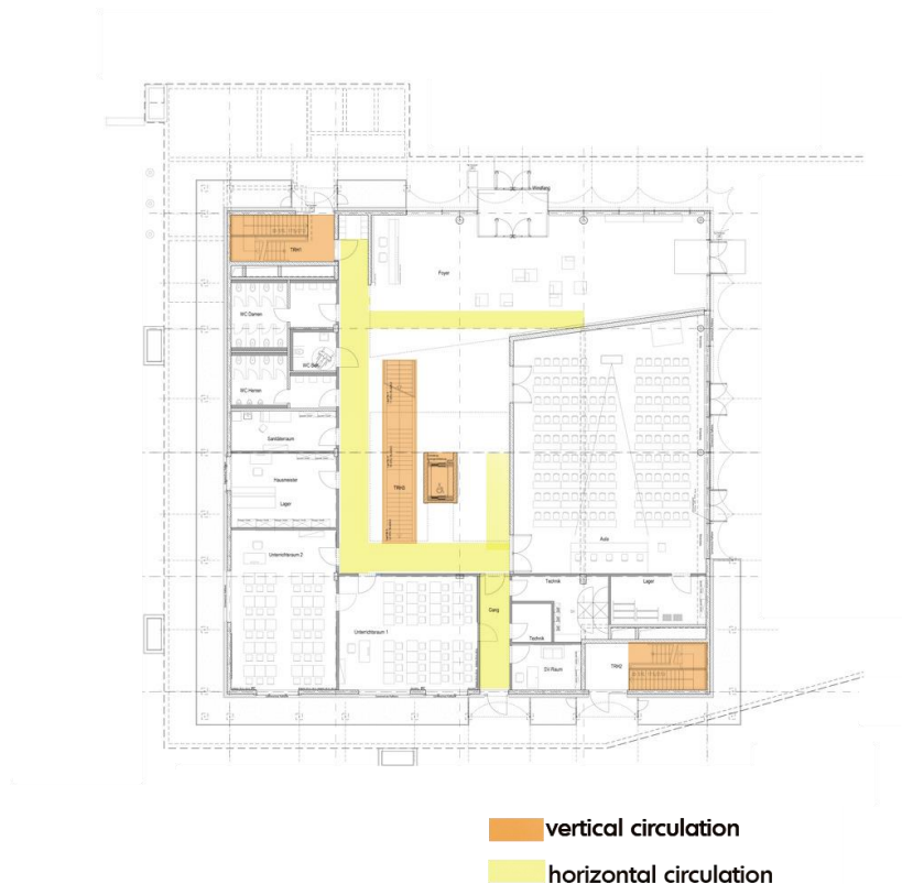
Figure 4.3 3Vertical and horizontal circulation.
