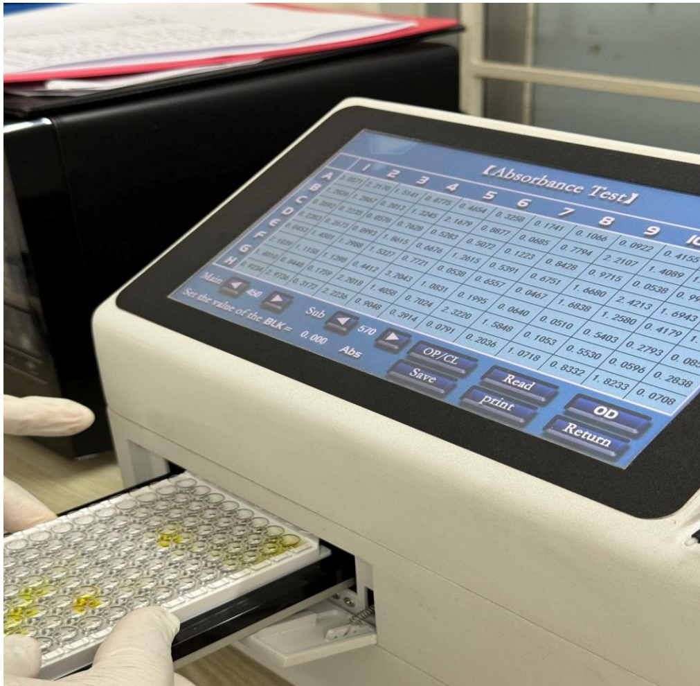
Figure 40: Measurement of Absorbance using Microplate Reader
