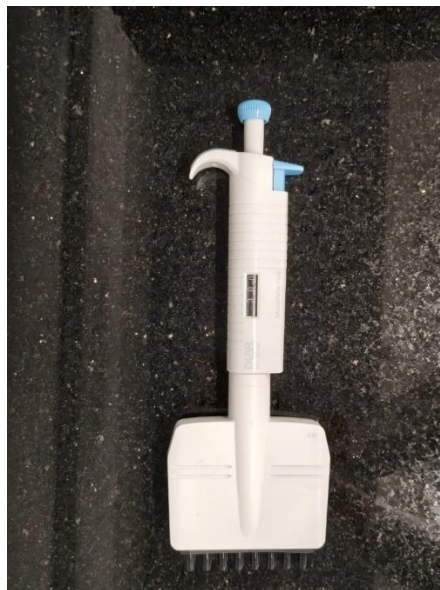
Figure 21: Multichannel micropipette (50 \mu L-300 \mu L)
