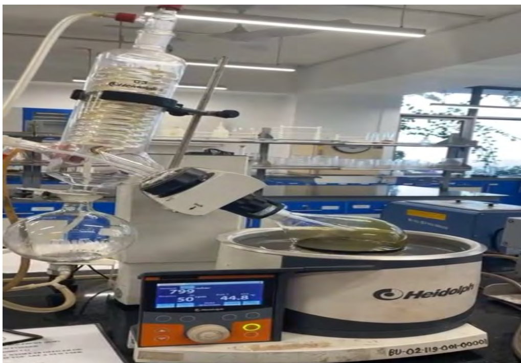
Figure-5: Evaporation through rotary evaporator in lab
