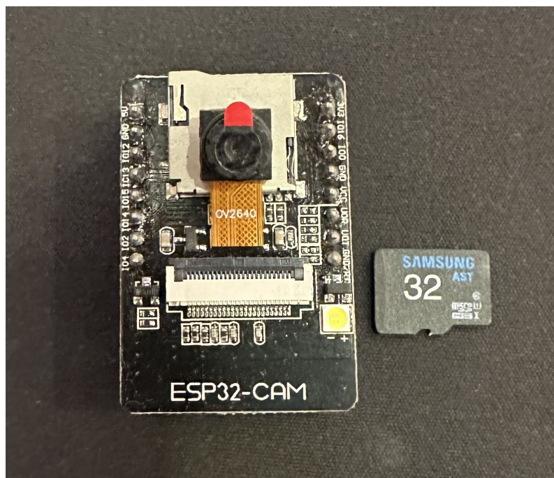
Figure 5.1: ESP32-CAM and SD card
