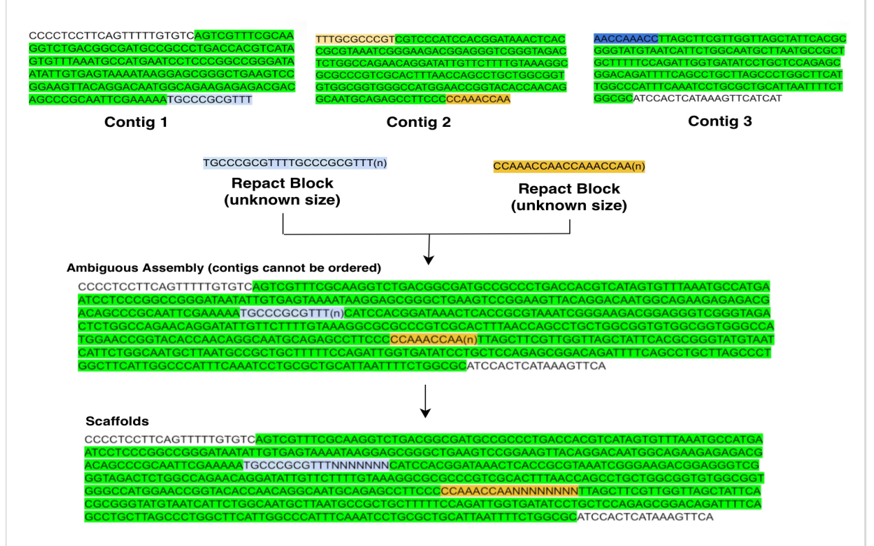
Figure 3.3: contig to Scaffold
