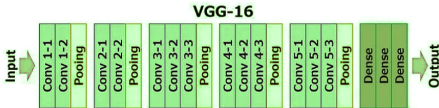
Figure 4.3: Architecture of VGG-16 model [14]
