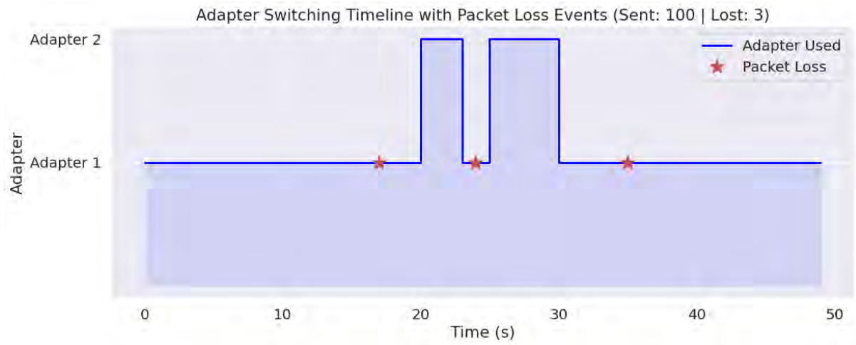
Figure 4.3.4: Adapter switching timeline with packet loss markers
