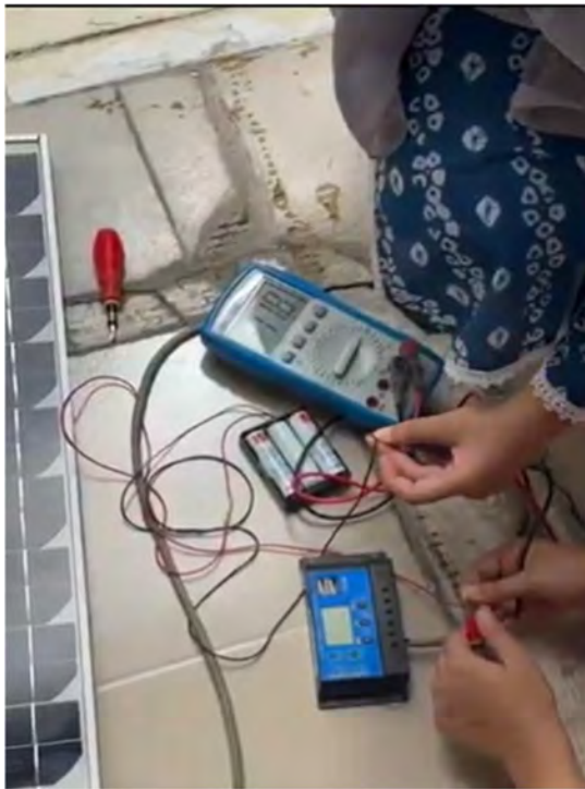
Fig 3.26. Before solar charging, battery charge= 11.8V
