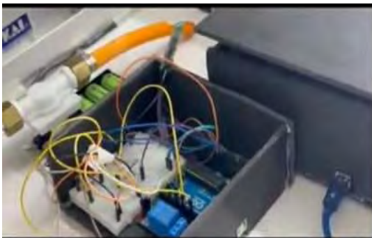
Fig 3.24. Solenoid valve is Open when gas is below 2000ppm
