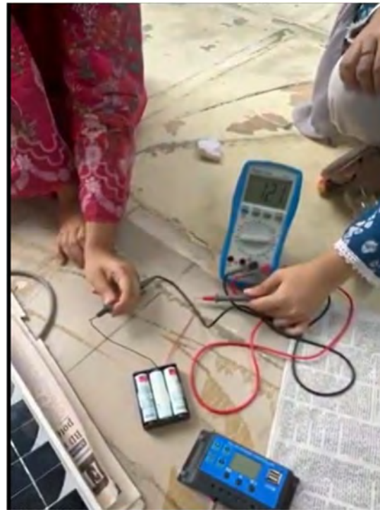
Fig 3.27. After solar charging, battery charge= 12.1V
