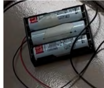
Fig 3.14. 12V Lithium-ion battery
