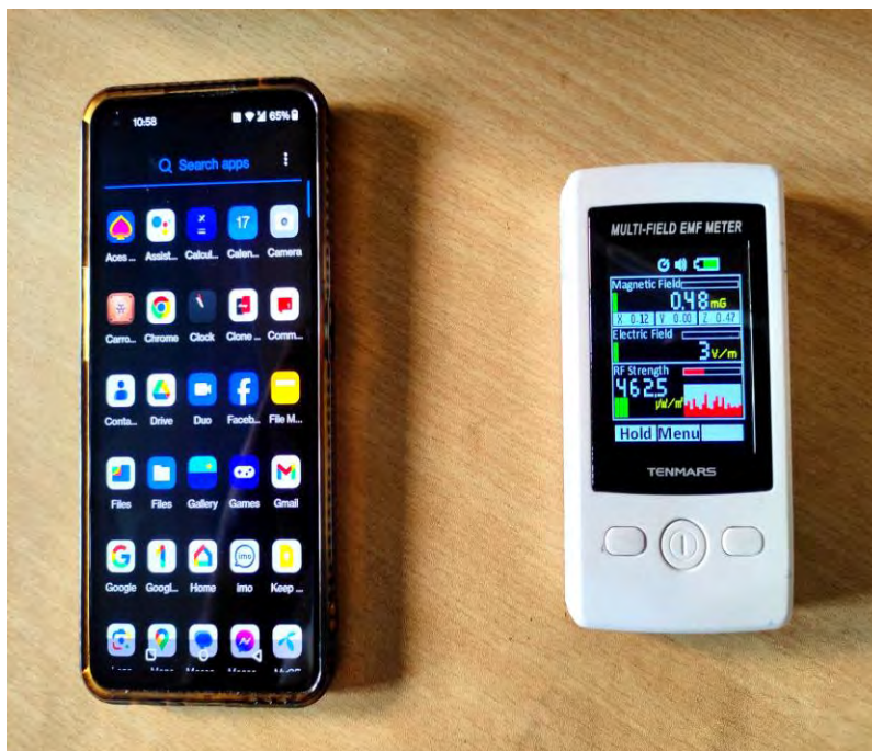
Figure 02: Multifield EMF Meter.
