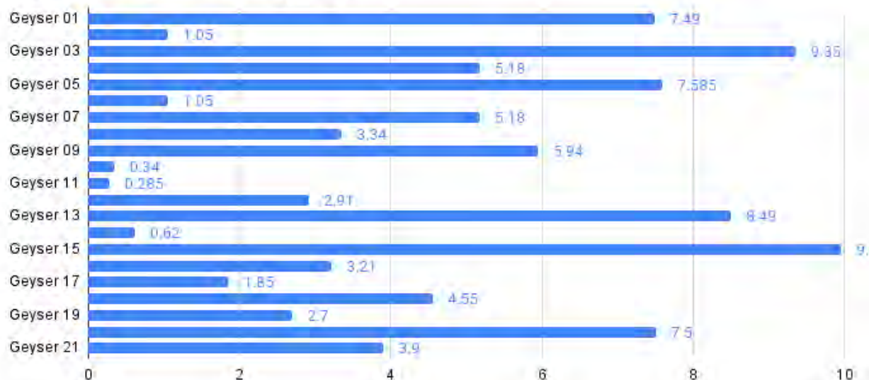
Figure 112: Geyser Magnetic Field (mG) Bar Chart
