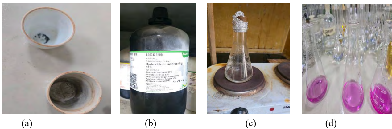
Figure 11. Procedure for determination of alkalinity (%) of ash of pectin: (a) ash sample obtained after incineration, (b) addition of 25 mL HCl solution, (c) gentle boiling of HCl solution, and (d) endpoint detection using phenolphthalein indicator with colour change from colourless to pink during titration.
