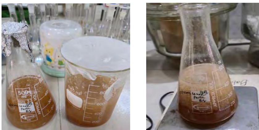
Figure 16. Precipitation of pectin after addition of alcohol
