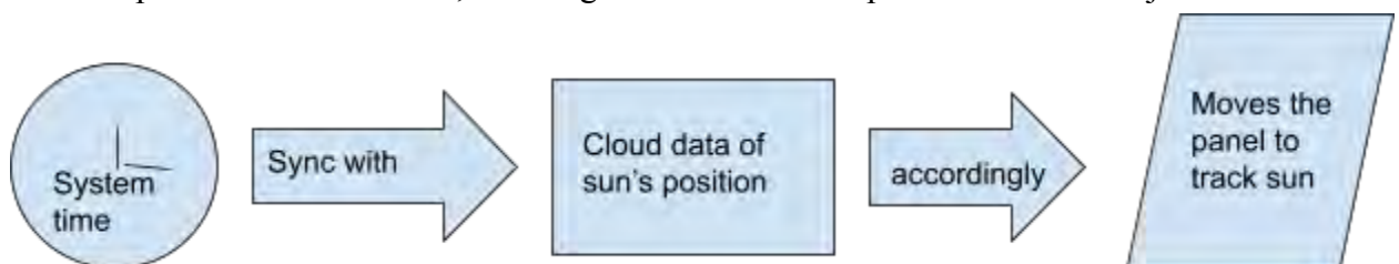
Figure 2: Time Based System Algorithm
