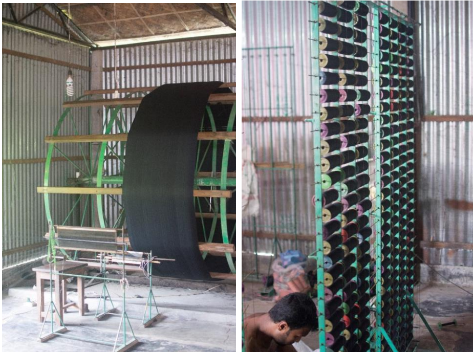
Figure 8.5: Thread Warping Machine present in Pathrail, Tangail
