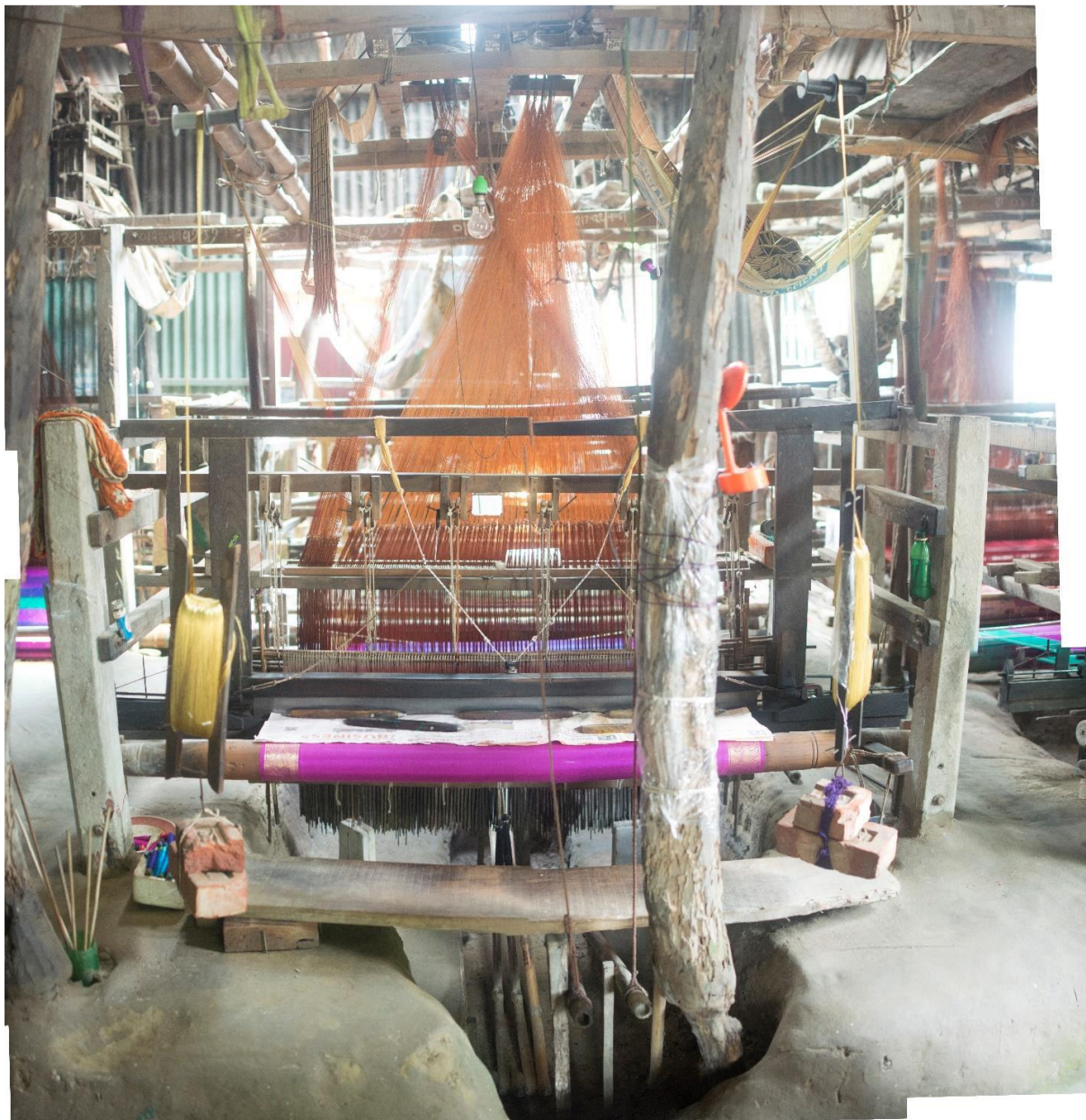
Figure 5.4: Traditional Pit-loom machine with Jacquard Weaving
