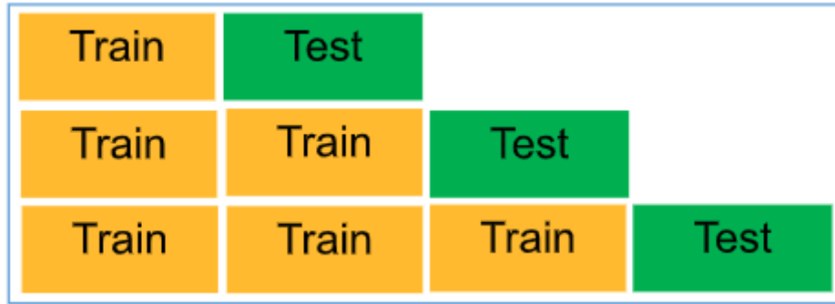
Figure 3.7: k=3 fold cross validation scheme
