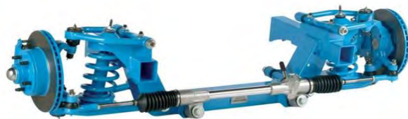
Fig: 3.1.2b Independent Suspension System
