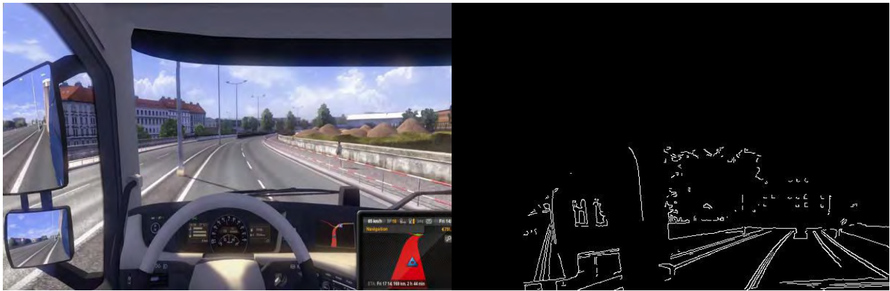
Fig: 4.2.1c. Canny Edge detection output
