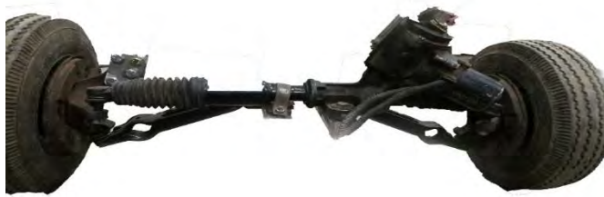
Fig: 3.1.4 Electric power steering in our system
