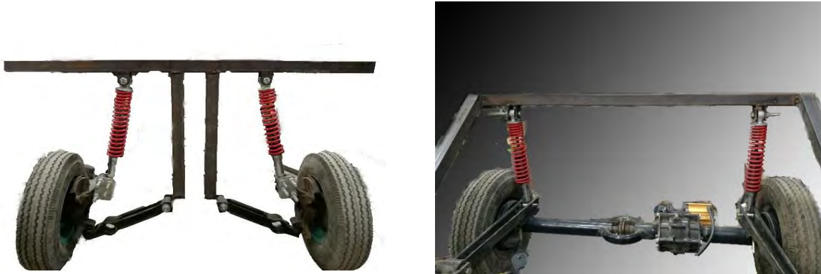
Fig: 3.1.2c Front & Rear Suspension mechanism of our mechanism
