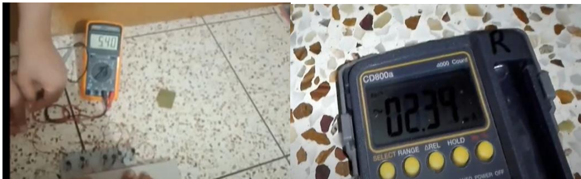
Figure 11: Voltage and Current from Piezo mounted under tiles
