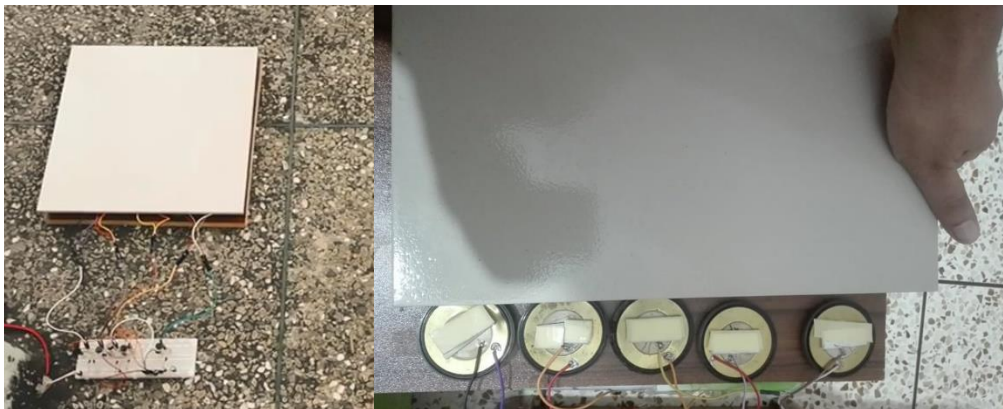
Figure 8: Piezo Mounted under tiles
