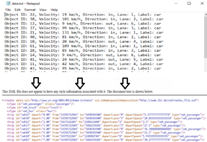
Figure 5.9: Vehicle detection output to trips.xml conversion
