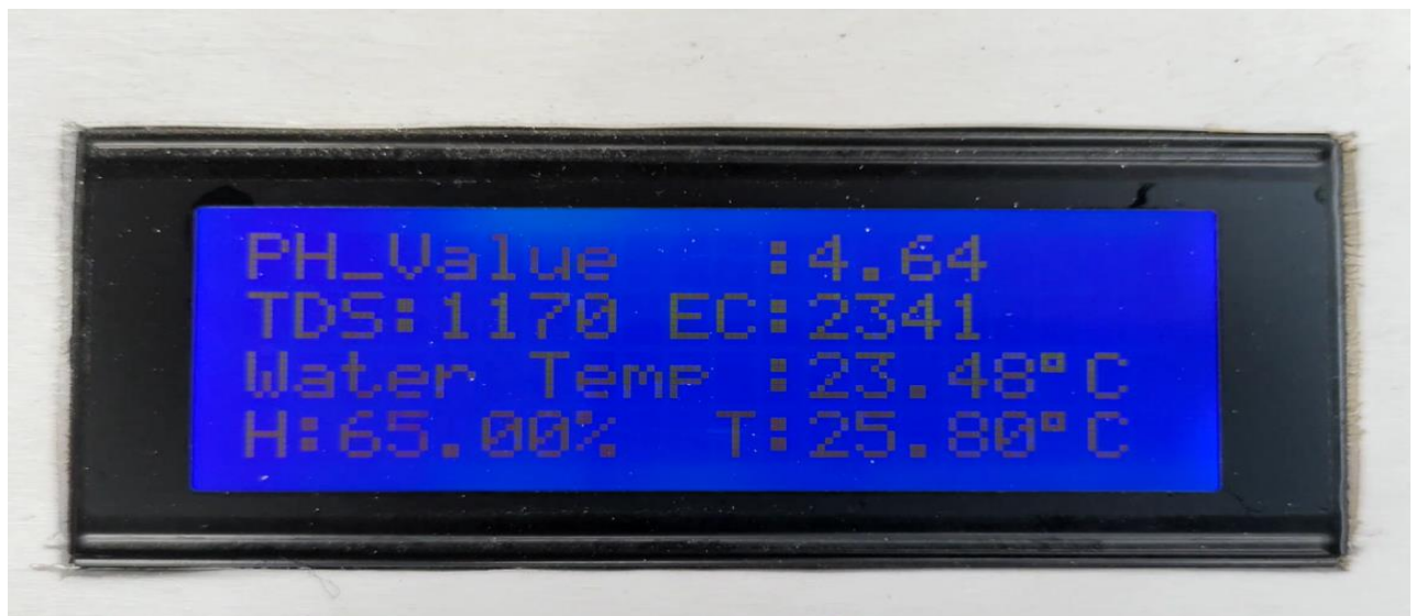
Fig: 5.3.2 TDS value of the LCD IS 1170 where the meter is showing 1260
