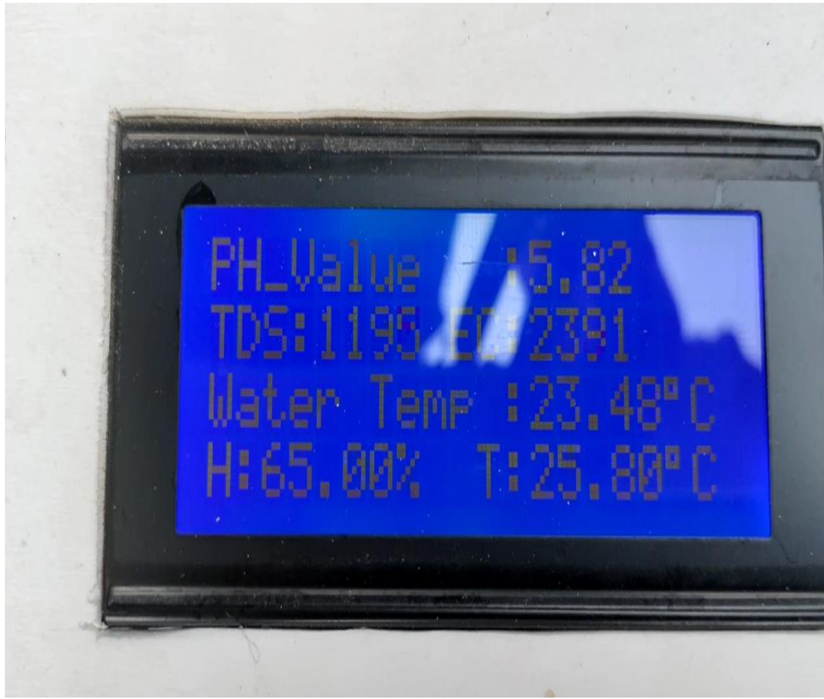
Fig: 5.3.1 from the above figures we can see the validation of the pH sensor of our system. The pH of the coffee solution is showing 5.41 and, in the LCD, it is 5.82.
