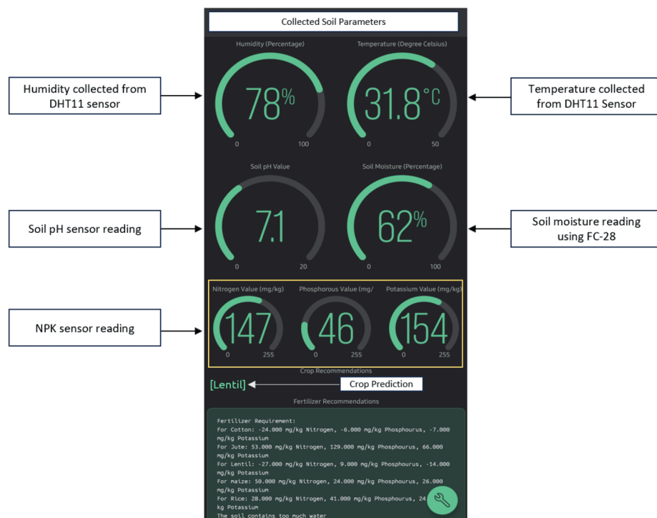
Fig 18. Displaying data collection and suggestions in the Blynk IoT mobile application interface.
