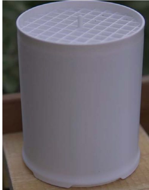
Fig 5.2.1.2- Post Assembly of the Tipping Bucket Housing and Internal Magnet-Lever Mechanism for Rainfall Measurement.
