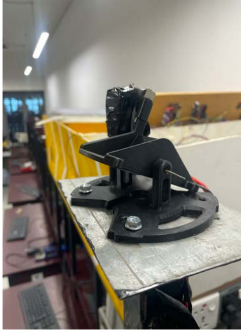
Fig 5.2.1.2- Post Assembly of the Tipping Bucket Housing and Internal Magnet-Lever Mechanism for Rainfall Measurement.
