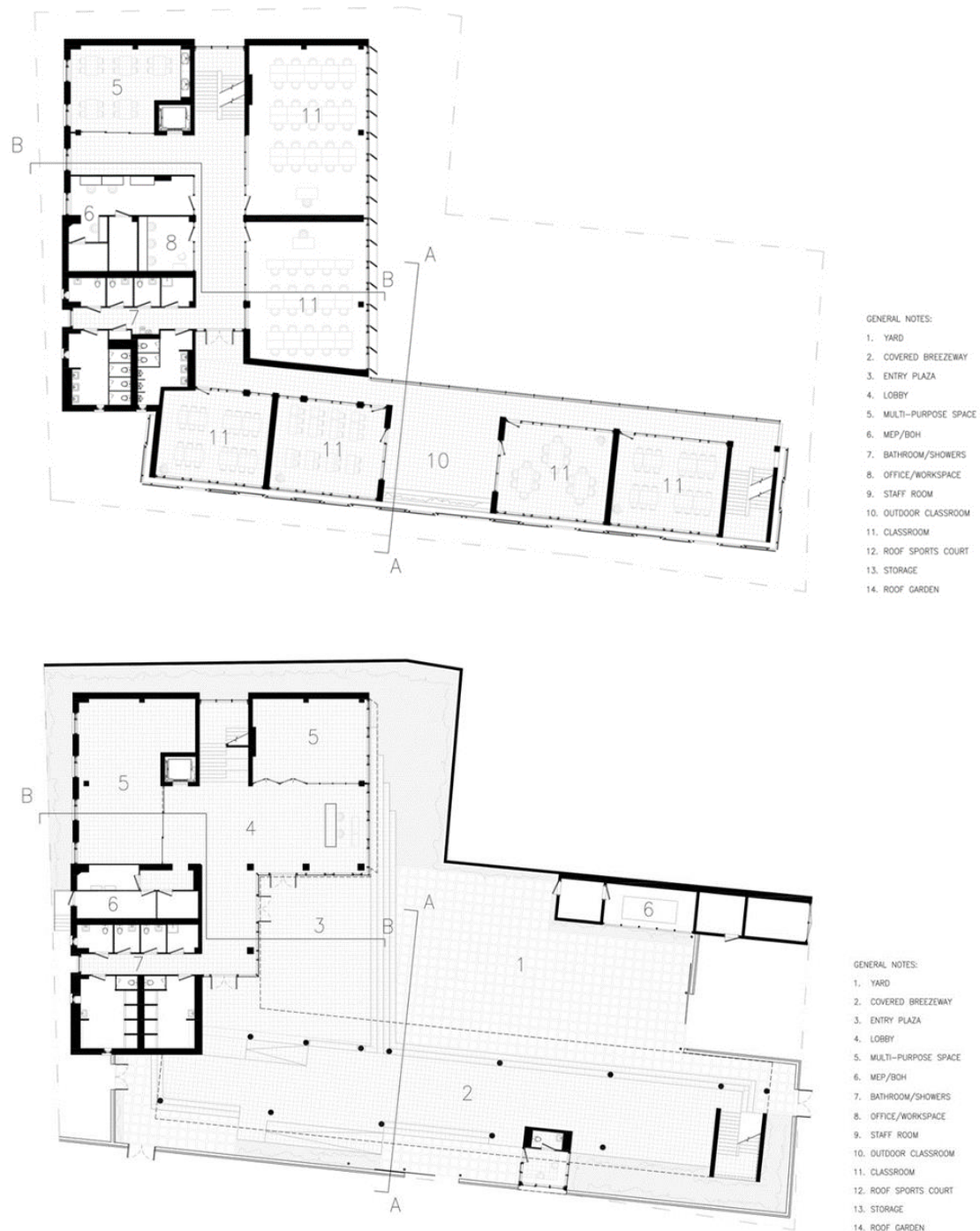
Figure 27: Plans show the large amount of open areas that are good for natural ventilation. Source: ArchDaily.com
