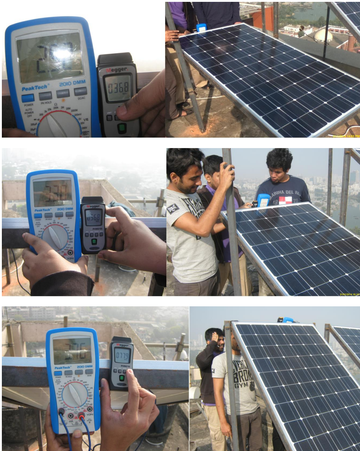
Fig 4.2: Short circuit current and irradiance for tilt angles a) 10^\circ , b) 23^\circ and c) 40^\circ
