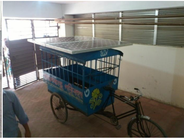
Fig 5.3: Tri-Wheeler Van with PV support
