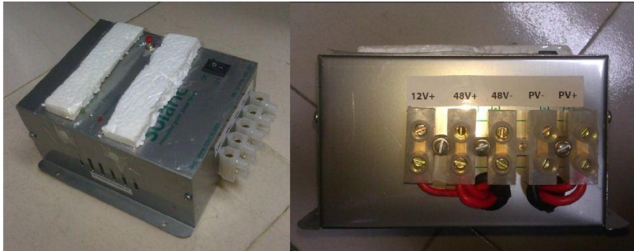
Fig 3.5: PWM Charge Controller
