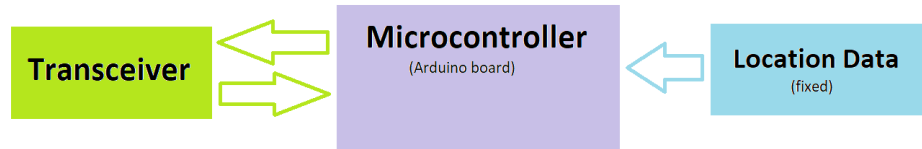
Figure 2.2: block diagram of infrastructure unit
