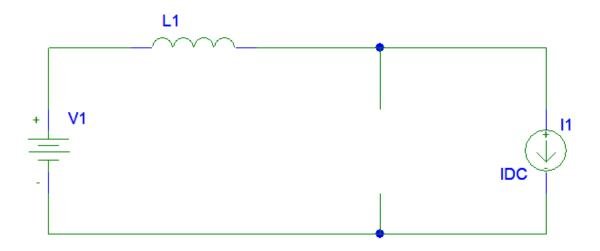
Figure 2.2(e): Switch Closed and D3 Off(t3<t<T)
