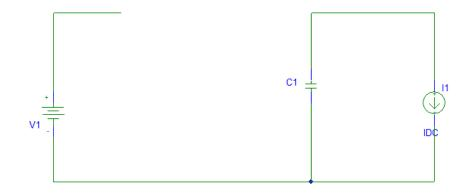
Figure 2.1(d): Switch Open and Diode Off
