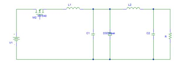
Figure 2.1(a): Resonant Converter with Zero Current Switching
