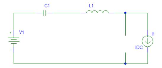
Figure 2.2(b): switch open and D1 off (0<t<t1)
