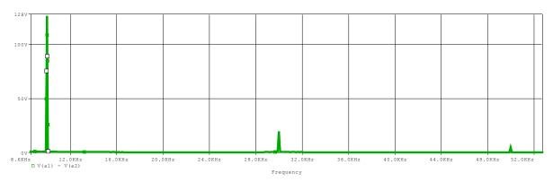
Figure 3.4(b): F.F.T of Wave Shape Across Inductor And Capacitor.
