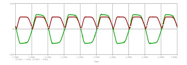
Figure 3.8(d): Combined Wave Shape of Inductor-capacitor & output.
