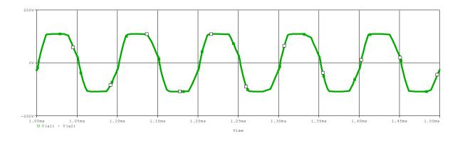
Figure 3.4(a): Wave Shape Across Inductor And Capacitor.
