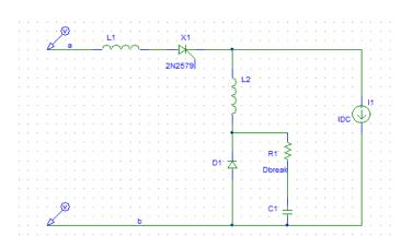
Figure 1.3(b): Diode Snubber Circuit
