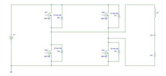
Figure 3.1:Series Resonant Dc-Ac converter.
