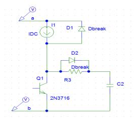
Figure 1.4(a): Turn On Principle Using BJT
