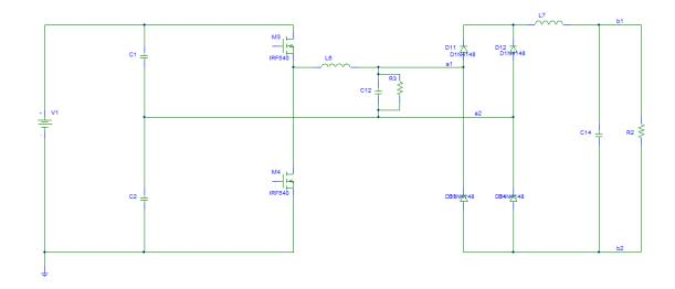
Figure 3.5: Parallel Resonant Dc-Dc Converter.
