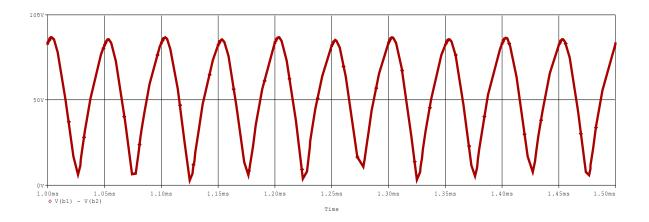
Figure 3.6(c): Output Wave Shape of Parallel Resonant Dc-Dc Converter.
