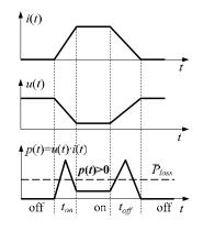
Figure 1.2(b):Power losses in real switches
