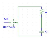
Figure 1.4(b): Turn Off Principle Using MOSFET
