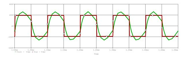
Figure 3.2(d): Series Resonant Dc-Ac Converter (input & output)
