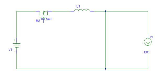
Figure 2.1(b): Switch Closed and Diode On  $(0 \le t \le t1)$
