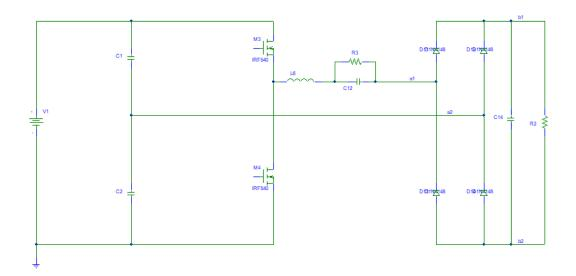
Figure 3.3: Series Resonant Dc-Dc Converter.
