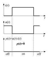
Figure 1.2(a):Power losses in ideal switches
