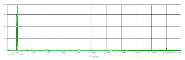
Figure 3.6(b): F.F.T of Wave Shape Across Inductor And Capacitor.
