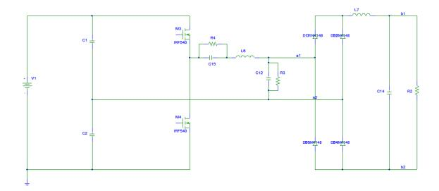
Figure 3.7: Series-Parallel Resonant Dc-Dc Converter.
