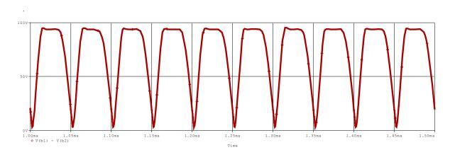
Figure 3.8(c): Output wave shape of Series-Parallel Resonant Dc-Dc Converter.
