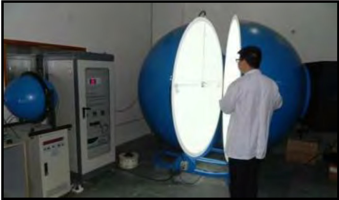
Figure 1: Commercial LED light testing using globe method.
