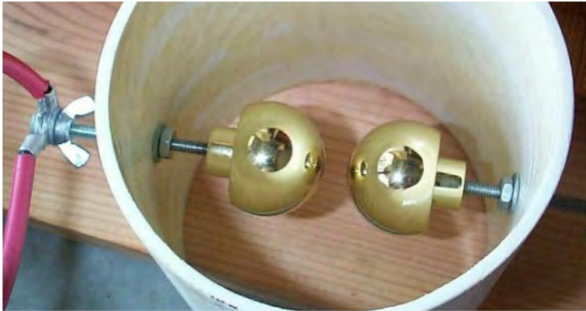
Fig. 4.7 Static spark gap [3]
