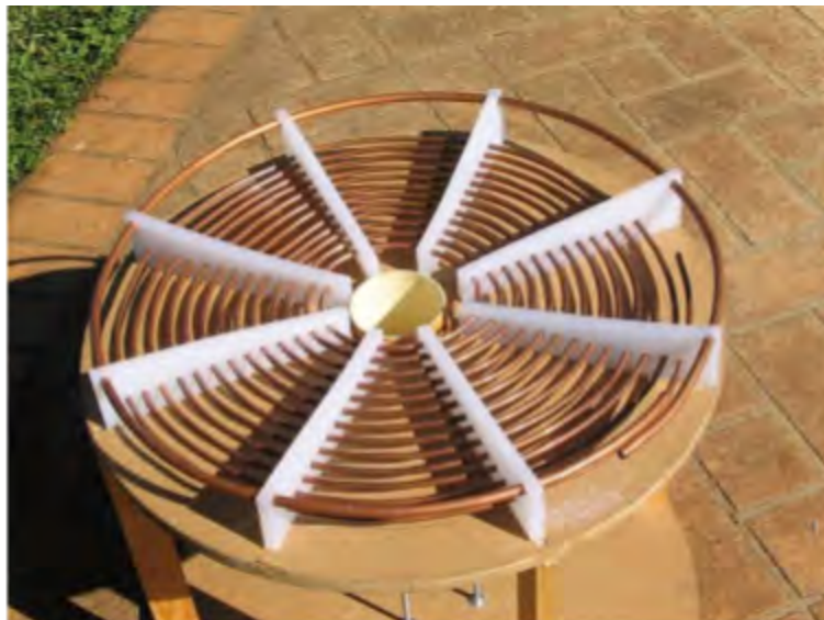
Fig. 4.4 Typical Primary Coil [3]
