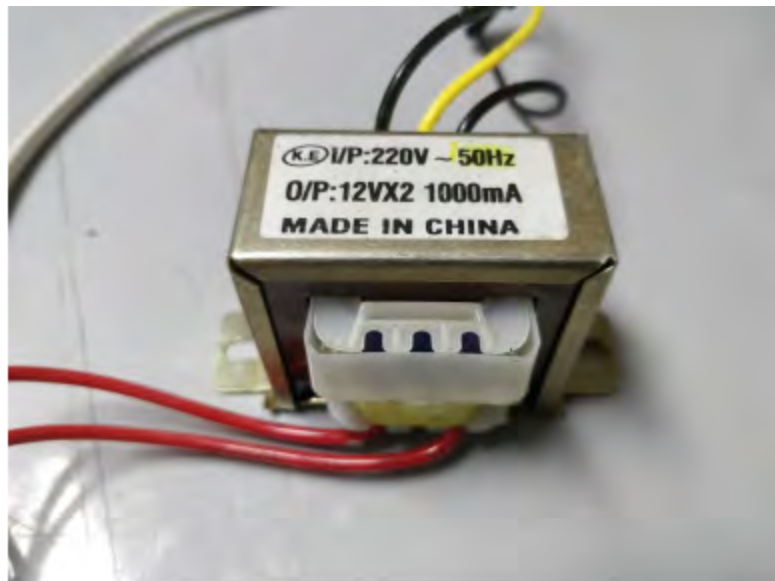
Fig. Step down transformer
