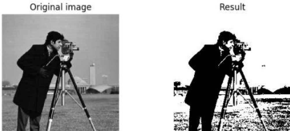
Figure 2.1-image before and after Thresholding [11]
