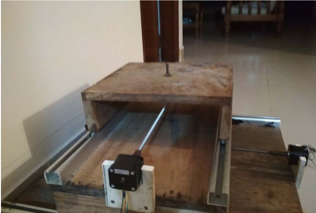
Figure 15: CNC machine with X and Y axis
