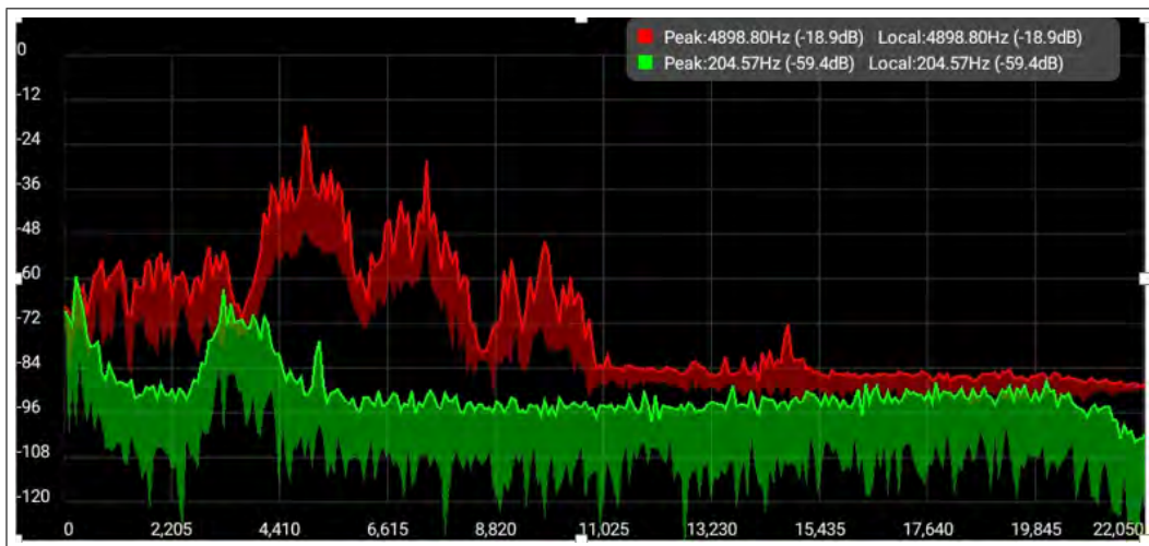
Figure 4.2: Received signal in frequency domain (Generated by Spectrum Analyze application)
