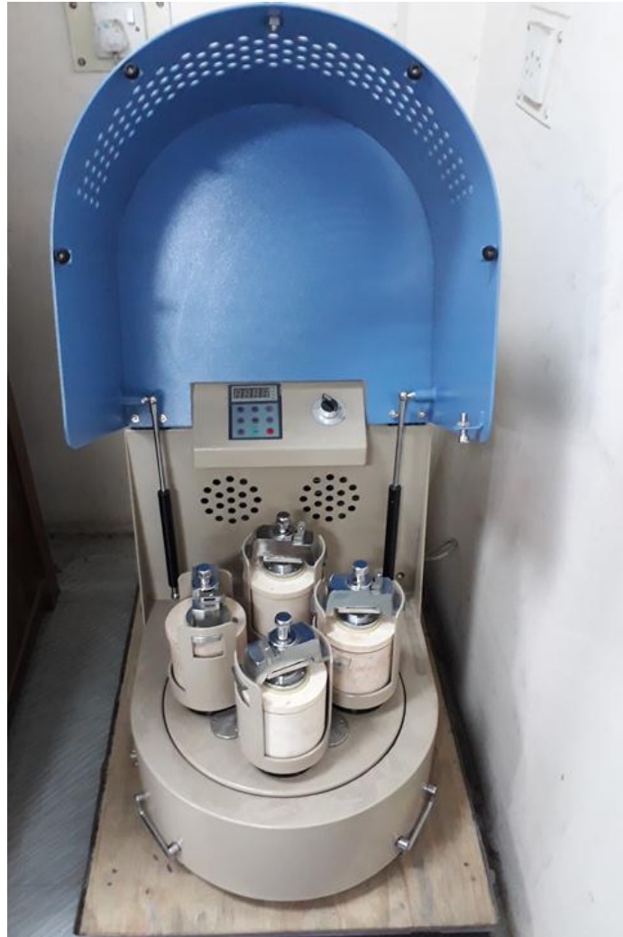
Figure 7: MSK-SFM-1 Bench-Top Planetary Ball Mill with cover opened
