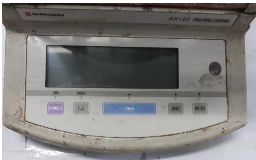
Figure 3: Control Fields and Display of AX120 Electronic Balance
