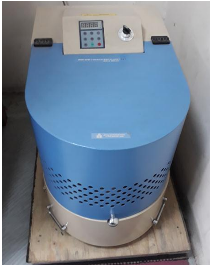
Figure 6: MSK-SFM-1 Bench-Top Planetary Ball Mill Machine
