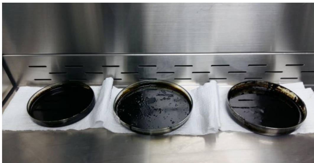
Figure 2.3: The petri-dishes containing the methanolic extract of L. aequata leaves placed under laminar air flow for drying.
