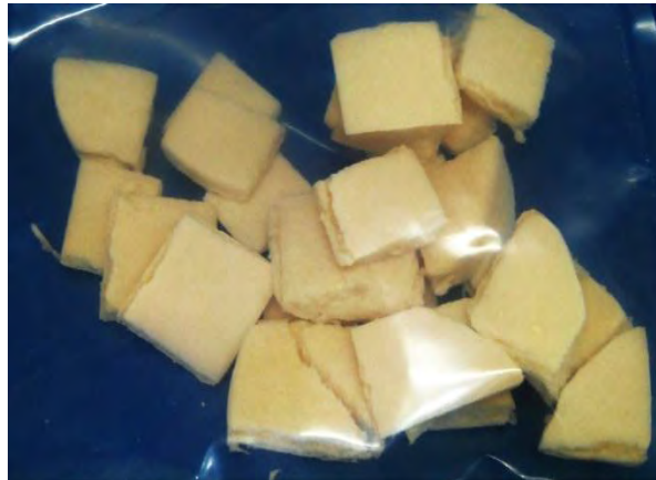
Figure 3.1: Fabricated scaffolds of HCA
