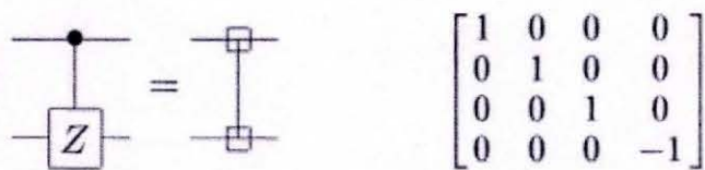
Fig 3.10 Circuit symbol and matrix representation of controlled-Z gate
