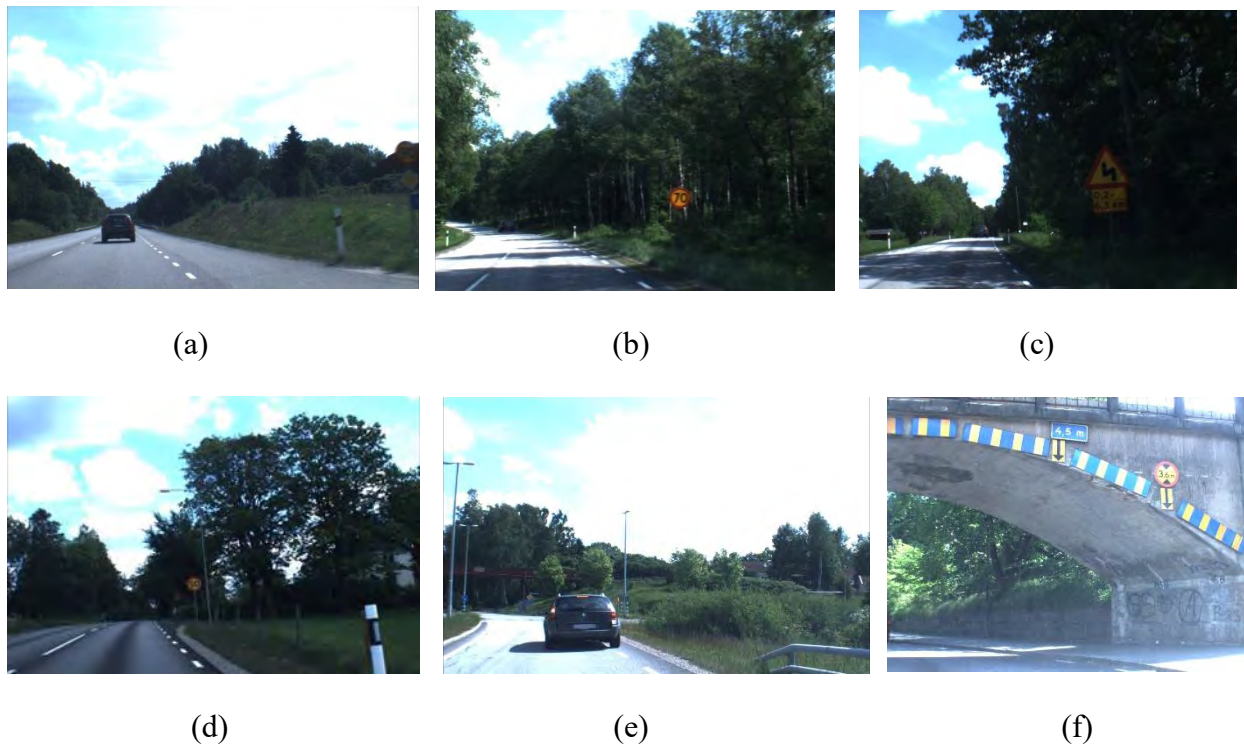
Fig. 2.3: Examples of some challenging scenes for a traffic sign detection system: (a) Motion blur; (b) Ocluded by trees; (c) Lighting variation; (d) Cloudy weather; (e) Sign hiding behind the car; (f) Similar background.
