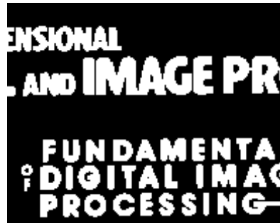
Fig 3.3 Opening: a 2 \times 2 square structuring element
