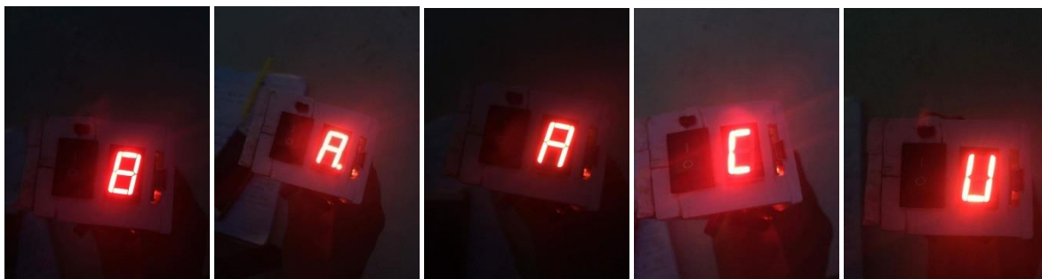
Fig 6.1.2:7- Segment display showing “BRACU” separately
