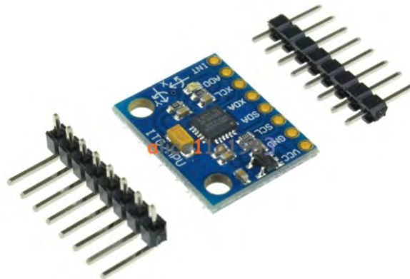
Fig 4.2.3: MPU 6050 Gyro Sensor
