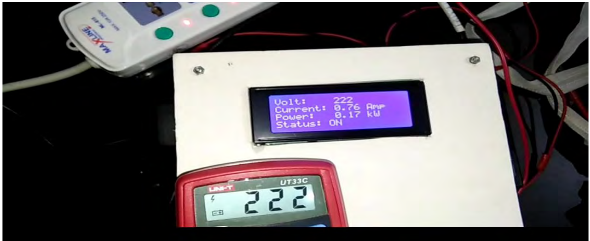
Fig: Status "On", Volt: 222 V, Current: 0.76Amp, Power: 0.17 KW
