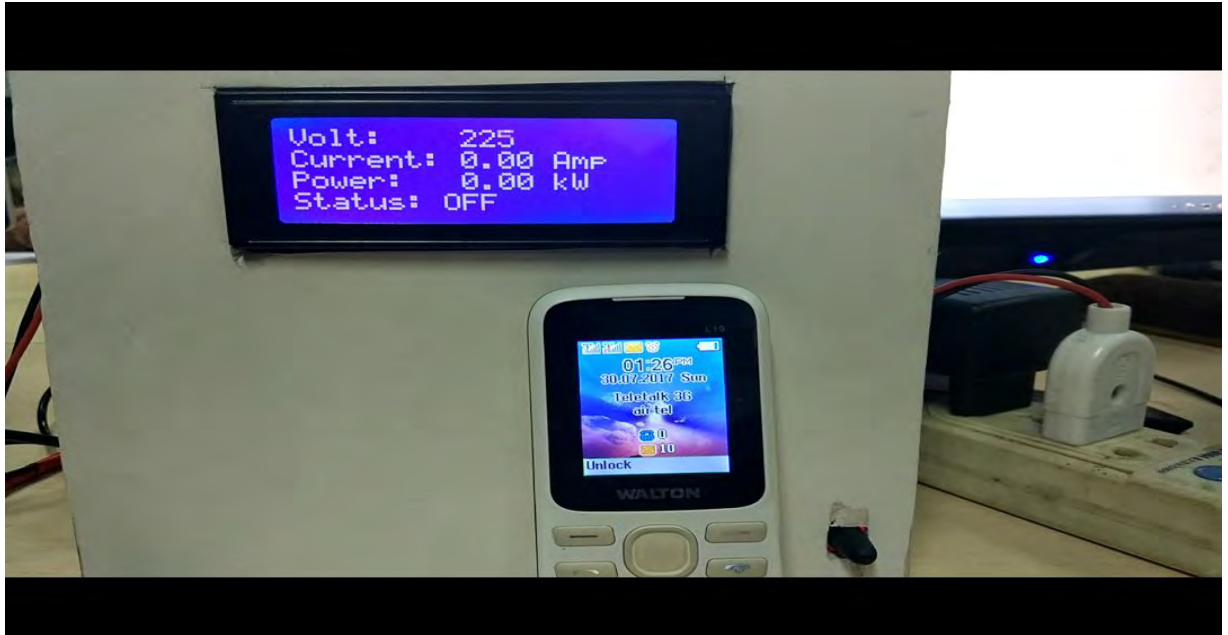
Fig: “Device Restarted” but Status is “OFF”
