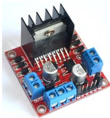
Figure 19: L298 Motor Driver
