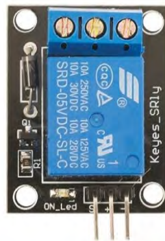
Figure 13: 5V Single Relay Board
