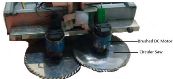
Figure 7: Brushed DC Motor and Circular Saw
