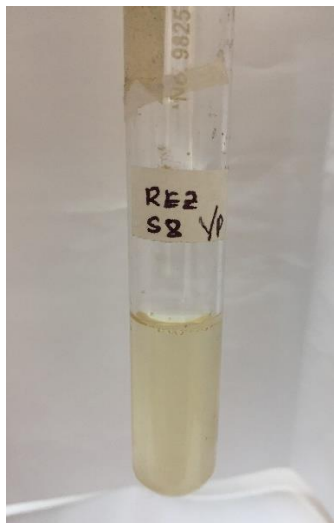
Fig 3.4 Negative result for the VP test showing no colour change upon addition of alpha-naphthol and potassium hydroxide
