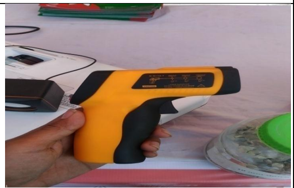
15.Laser thermometer for maintaining temperature.
