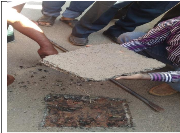
1. Sample collecting for proportion checking of Bitumen & stones.
